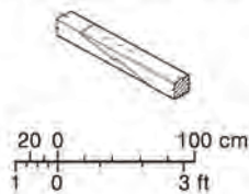
Scarf joint in collar purlin
